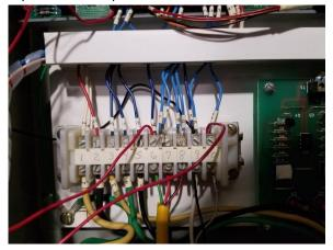
• Tie together remaining wires 7 and 8 to continue supplying ±1V to front panel dial and button
