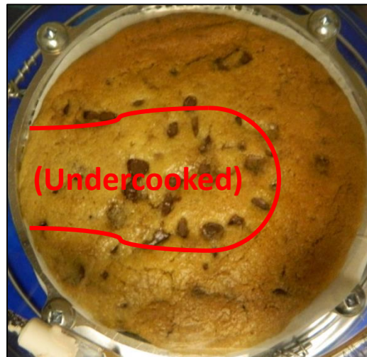
Figure 30: Top view of cookie baked with second baking enclosure setup with IR shielding (reduced undercooked region indicated)
